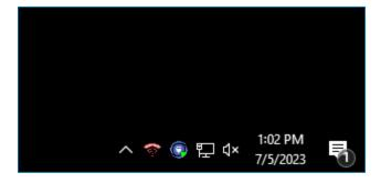
Right-clicking on the blue rThreat icon displays a window with the available manipulation options. The menu shows the control options of the software.
