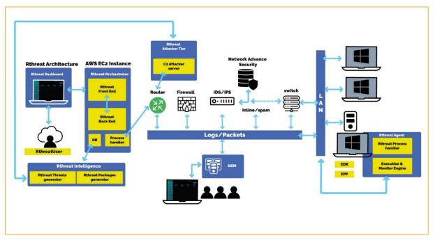
The rThreat artifacts contained in emulation packages are sent over the network and executed on the virtual machine (Endpoint) with the client's golden image. The rThreat Software applies control mechanisms and sends the response to the Orchestrator with the obtained results.
